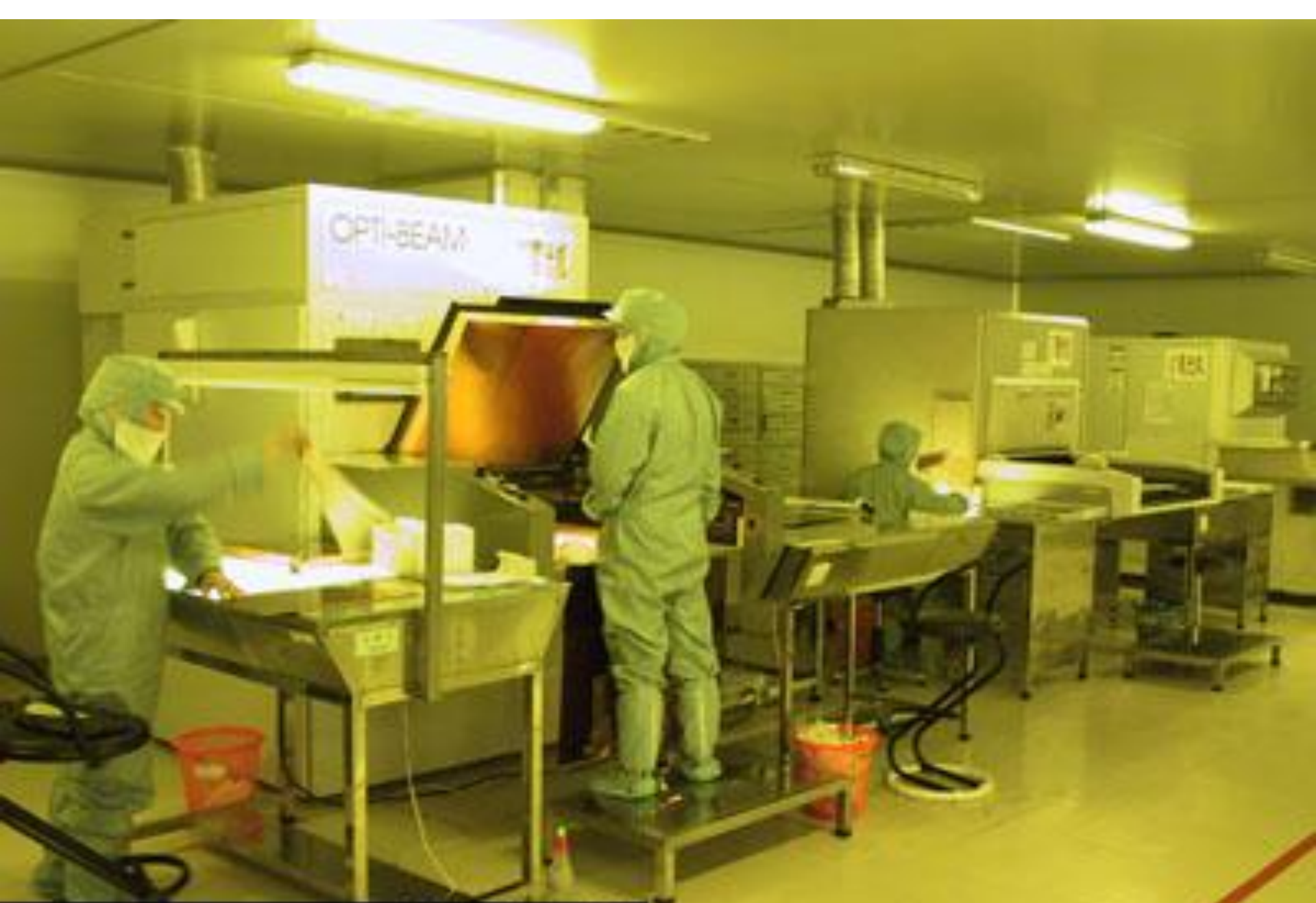
Dry Film Exposure 乾菲林曝光
