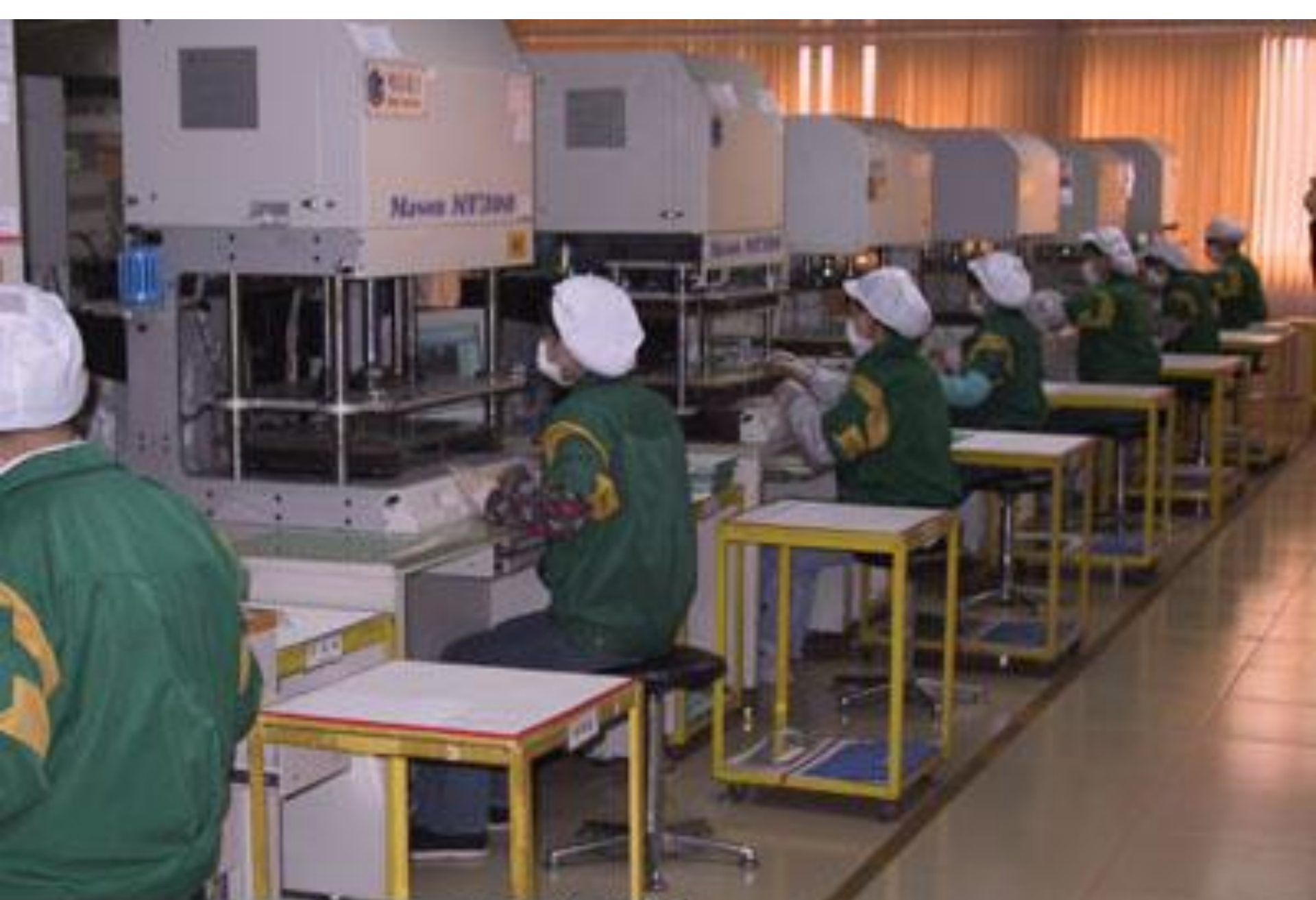
Open/Short E-testing 開短路測試
