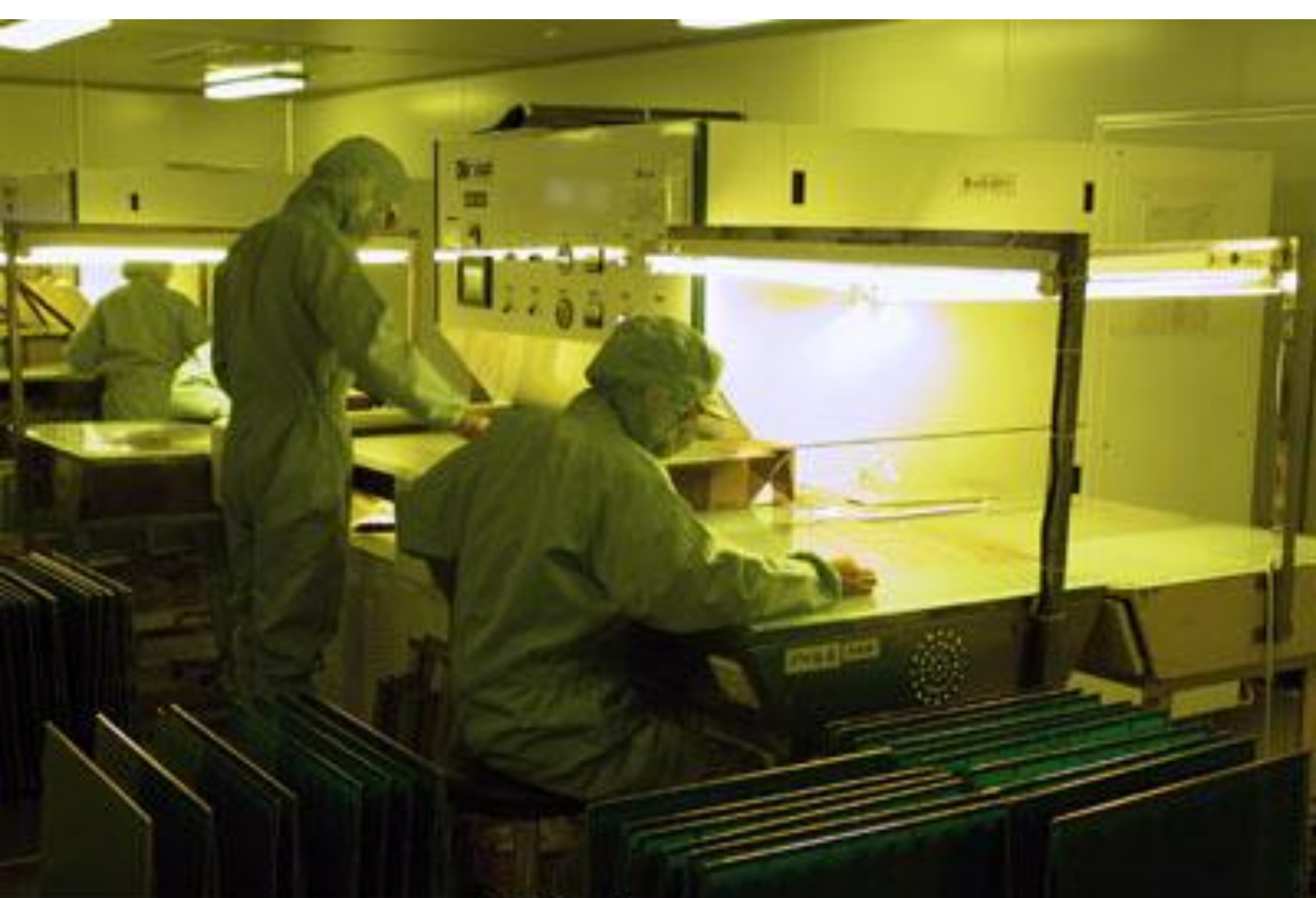
Wet Film Solder Mask 曝光綠油
